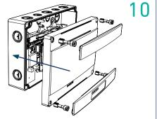
• Screw the lid to the backbox using the supplied plastic screws and refit top and bottom front plastics that cover screw housings.
